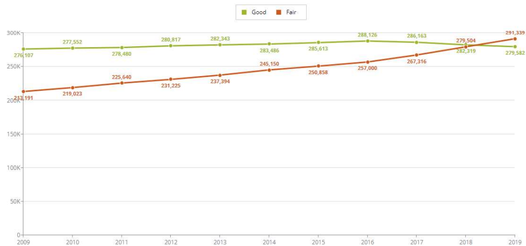
Figure 1.1: The structural condition, "good" or "fair", for the bridges across the United States between 2008 and 2019 (ASCE, 2021). For details on the description of structural ratings, please refer to table 1.2
