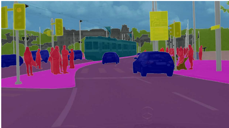
Figure 2.7: An example of semantic segmentation for an image showing street view and all the objects of interest segmented and assigned different colors according to their classes, (DWIVEDI, 2020)
