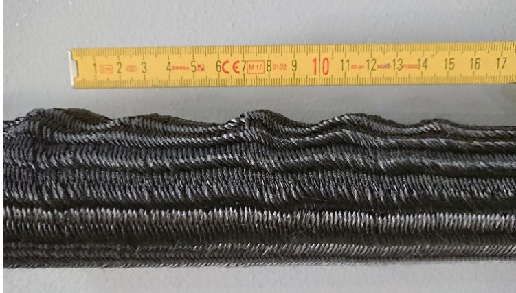
Figure 2-2: Loose braided hose consisting of n_{yarn} = 128 12k carbon fiber yarns at a braiding angle of \varphi = 60^\circ on a cylindrical mandrel with a diameter of d = 50 \text{ mm} ; wrinkles occur because the yarns cannot be compressed to the geometrically necessary width of w \approx 1.2 \text{ mm}
