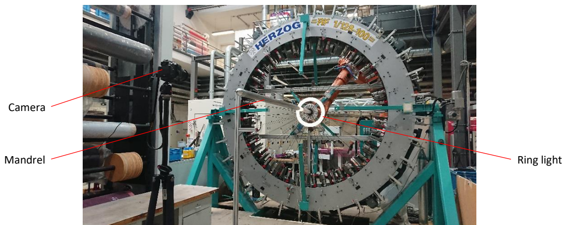
Figure 3-50: Arrangement of the camera at the side of the unbraided mandrel and of the ring light as backlight illumination behind the braid formation plane of the RF 1/128-100 braiding machine; illustration adapted from own publication [89]
