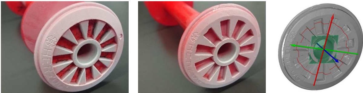
Figure 3-11: Notched area at the bottom of a bobbin (usually in contact with the locking pin; left); notched area at the top of a bobbin (turned down and usually not in contact with the locking pin; middle); 3D scan of the notched area shown in the middle with circular cross section drawn-in as a thin red line (right)
