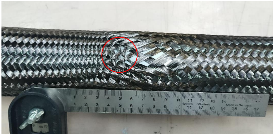
Figure 2-5: Hole in braided preform due to entangling of frayed fibers during formation of a spider's web; spider's web still visible as thin zigzag thread between the braiding yarns (marked with red circle)
