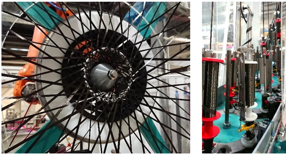
Figure 3-26: Sensor integrated braiding ring for measuring resulting radial forces fitted into the RF 1/128-100 braiding machine at the Chair of Carbon Composites (left, image taken from own publication [88]); screw-on barrel tensioner added to a bobbin carrier for replication of a yarn tension anomaly (right, image from own publication [89])
