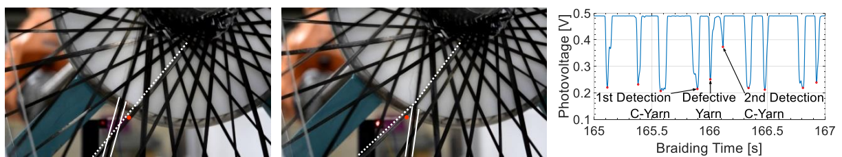
Figure 3-48: Still images during braiding at \varphi = 60^\circ and an elevated yarn tension of \sim 35 N of a single yarn (left and middle); yarn with elevated tension marked by two solid white lines; clockwise yarn that is detected twice marked by a white-dotted line; note the kink of the yarn/the white-dotted line in the image in the middle; for reasons of a better visibility of the laser light on the carbon yarns, it is drawn-in manually by a red dot; corresponding measurement reading from the photodiode (right)
