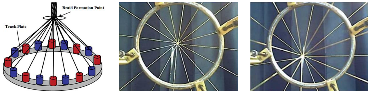
Figure 2-11: Schematic of an axial braiding machine including the braid formation point (left); braid formation point in the center of the camera view during regular braiding (middle); braid formation point deviating from the center of the camera view during defective braiding (right); images taken from [70]
