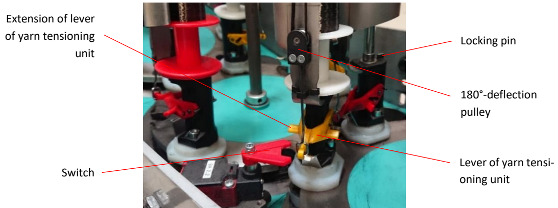
Figure 2-8: Switch for braiding process interruption and yarn tensioning unit of a bobbin carrier with lever; image taken from own publications [64,65]
