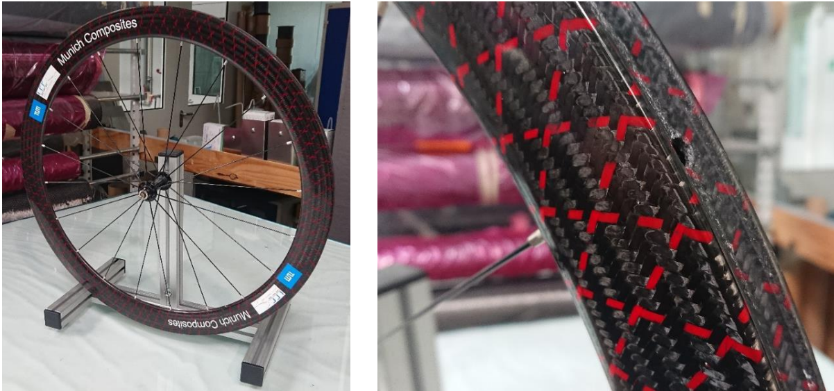
Figure 1-4: Braided bicycle rim developed within a joint research project between the Chair of Carbon Composites at Technical University of Munich and Munich Composites GmbH (overview left, close-up right)
