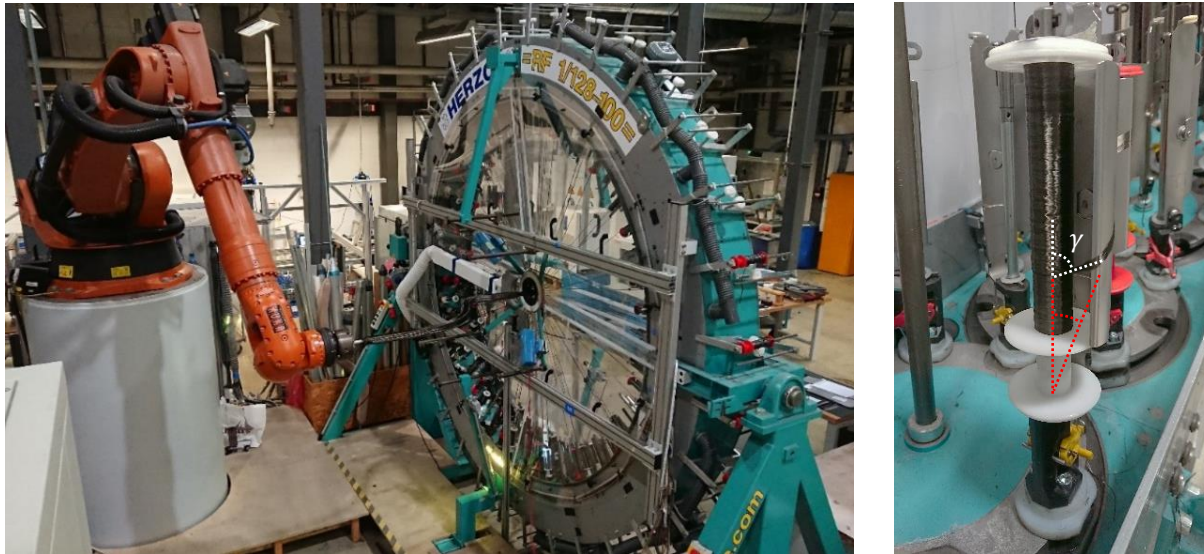
Figure 1-3: Radial braiding machine RF 1/128-100 with mandrel guidance by robot (left); IFDA-100 carrier with guide plate optimized for low fiber damage during processing of brittle reinforcement fibers as well as modified bobbin with unused bottom in order to avoid acute angles during unwinding of the yarn (right; actual unwinding angle \gamma drawn-in as white dotted line, acute but avoided unwinding angle drawn-in as red dotted line)
