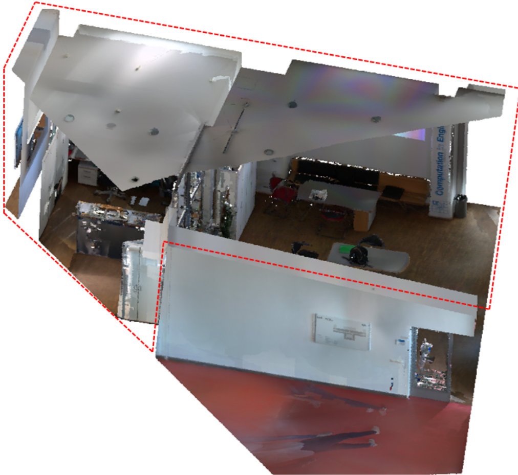
Figure 7: Top view of visible points at camera position in Figure 6. Points behind the wall (within the red dash line) are actually not visible from the camera pose.
