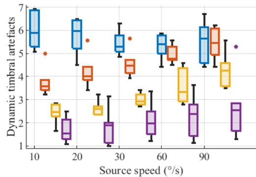
**Figure 2:** Median and quartiles of the dynamic timbral artefacts ratings for the regular panning methods at different angular source speeds. Blue: NLS; red: VBAP; yellow: PEP; purple: Higher-Order Ambisonics.
