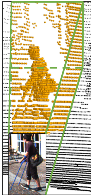
Figure 2.6: Extracting frustum point cloud. Green lines represent the frustum of the given 2D image cropped into the 2D bounding box of the pedestrian. The orange points represent the points that reside inside the frustum.
