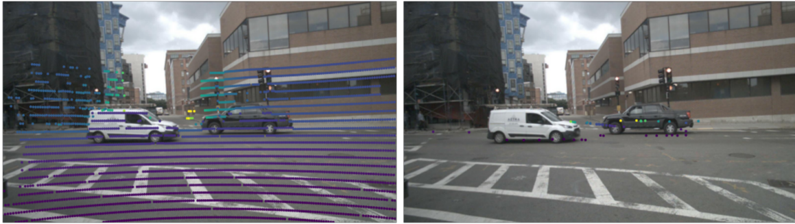
Figure 2.4: Lidar (left image) and radar (right image) points clouds projected onto the image plane of a scene in the nuScenes dataset [Cae+20]. The point colours indicate the depth values.
