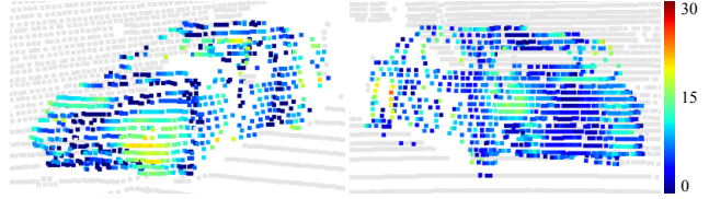
Figure 11. Color-coded deformations in cm learned by the proposed method. The perturbation does not affect every point, its magnitude is relatively low, and local smoothness is preserved.
