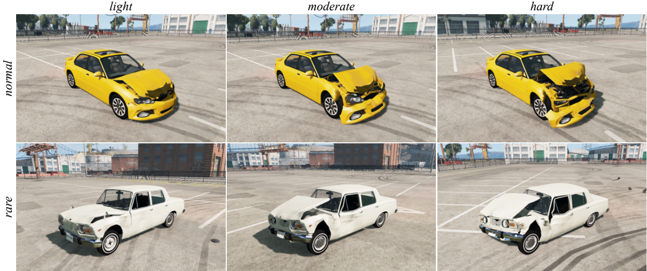
Figure 7. Comparison of linear damage intensities for normal and rare cars of CrashD. For each type of car, the accidents were created by the same hitting vehicle, coming from the same angle. It can be seen that the hard crash compromised the structure of the weaker rare car, while the normal car absorbed the impact differently, leaving the cabin unchanged.
