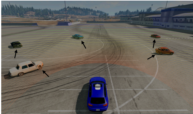
Figure 6. LiDAR scene setup of CrashD. For each car, a black arrow indicates its damaged area, which is ensured to be visible from the sensor viewpoint. Image used with courtesy of BeamNG GmbH.
