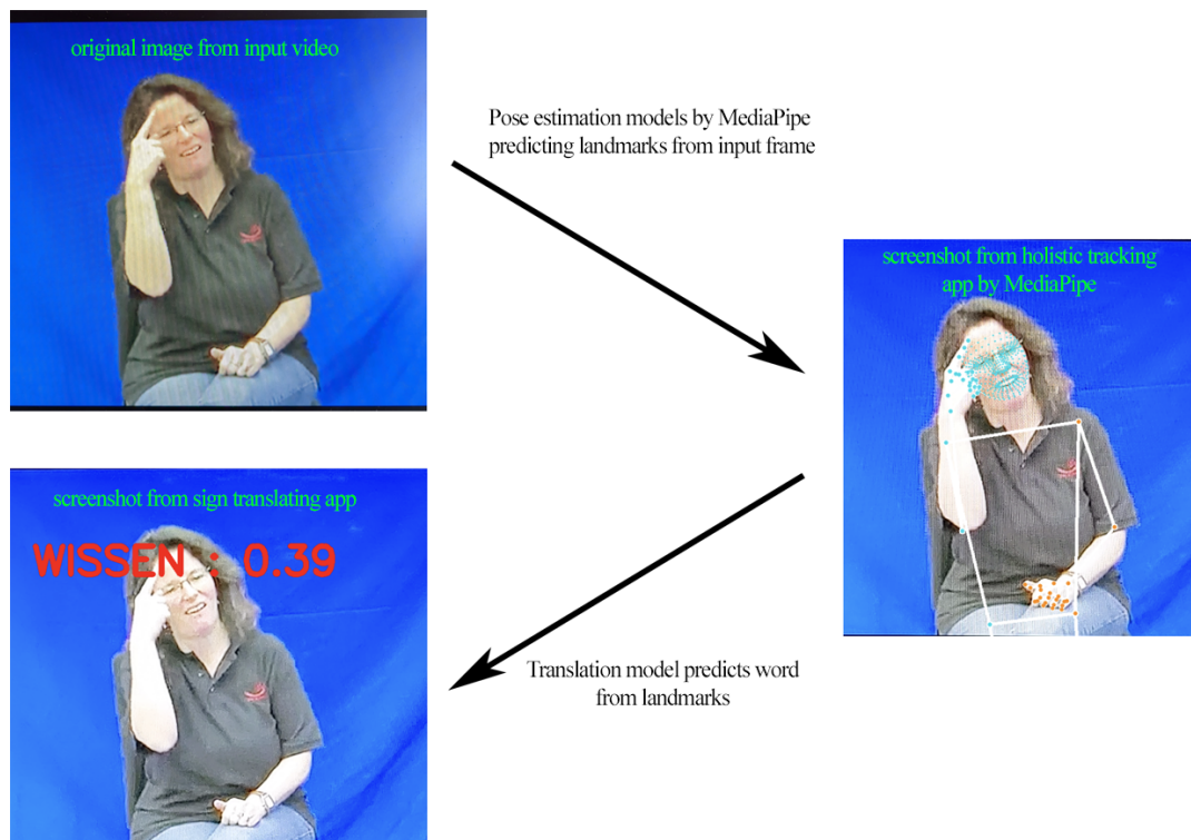
Figure 1.2.: Dataflow from input image to landmarks to translated sign.
