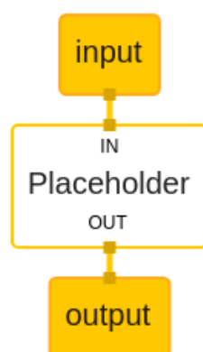
Figure 3.11: Basic MediaPipe graph with a placeholder for one calculator node.
