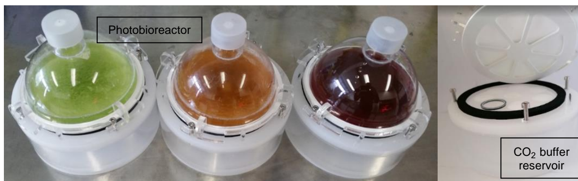
Figure 20: Photobioreactor HDC 1.100B for the cultivation of H. pluvialis at different cell stages [9].
