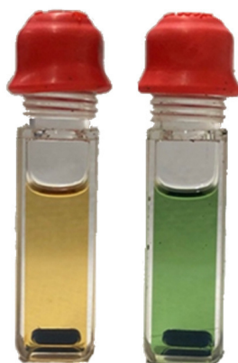
Figure S55. UV-Vis cuvettes with a solution of 1 - after the deprotonation using \text{KO}^t\text{Bu} (left), and before the deprotonation ( 1-H , right). The yellowish color of 1 - is a concentration effect, in higher concentrations 1 - is deep red.
