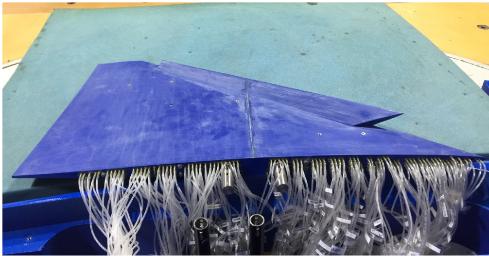
Figure A.6: The lower surface of the Model56 wing showing the silicon tubes of the pressure measurement probes for the connection to the acquisition system.
