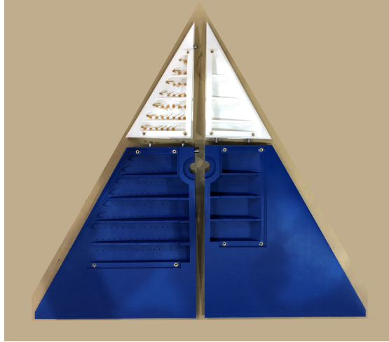
Figure 4.5: DW60 wind tunnel model seen from below, showing the hollow portions for the tubes accommodation and the interconnections for the final assembly.
