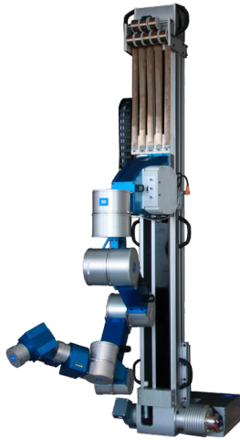
Figure 4.9: Our sweet pepper harvesting robot CROPS in 9 DOF configuration [215].
