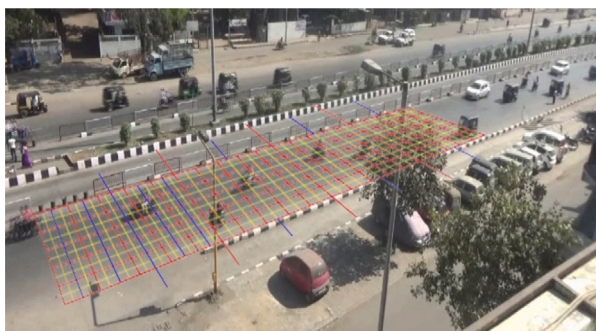
Fig. 4. Grid overlaid over the captured video data of the mid-block crossing area (Golakiya and Dhamaniya, 2018).
