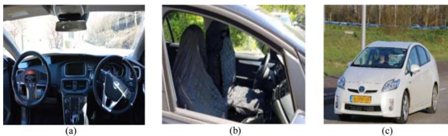
Figure 2 .#Examples of the WoZ technique. (a) Dummy steering wheel with no function for the driver (Habibovic et al., 2016), (b) Seat cover used to hide the driver (Fuest et al., 2018), (c) In-vehicle controller with an inactive driver (Palmeiro et al., 2018).
