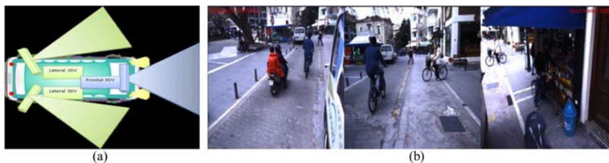
Figure 3 .#Example of data collection in a road trial of CityMobil2 shuttles. (a) The positioning and area covered by three 3DV cameras, (b) Example of a road scene displayed by three 3DV cameras. Source: (Madigan et al., 2019).
