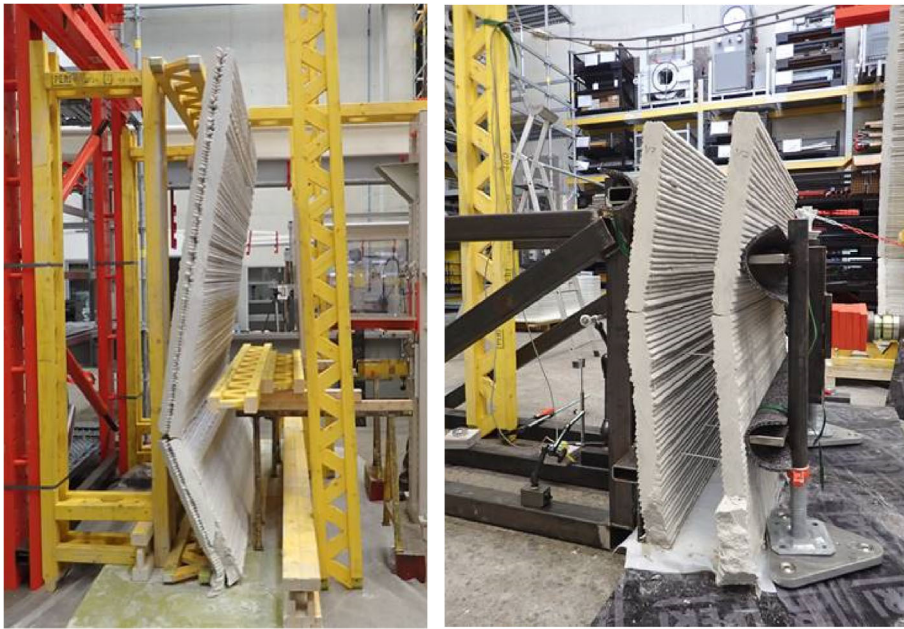
FIGURE 3 Approval tests for material certifications (ZiE) for 3D-printed concrete components, carried out at the TU Munich (pics: D. Weger)
