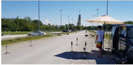
Figure 5: Experimental setting: subject standing next to the street, wearing the HMD with virtual vehicles approaching.
