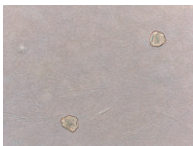
Figure 9: Microscope picture of birch pollen deposited on the bottom of the prototype chamber. (400X magnification). The birch pollen looks wrinkled due to natural drying of water containing pollen (i.e. this is how pollen flies in ambient air: wrinkled).
