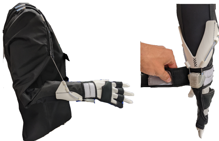
Figure 5: Elbow exosuit prototype developed at the LfE with two actuated and linked cables running in parallel.
