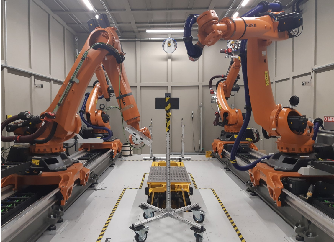
Figure 9.1: Robotic CT system ("RoboCT") of the BMW AG. The setup for this work comprises two cooperative robots carrying the detector (left) and the source (right) as well as a mobile sample holder (middle). The latter is equipped with an X-ray transparent polystyrene block at the top on which the test part (see fig. 9.2) was fixated. Only the two robots in the foreground were used for this investigation.
