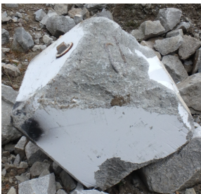
(b) Photograph of the impacting object T092 (some damage can be observed). The visible metal cap covers the housing of the motion sensors.
