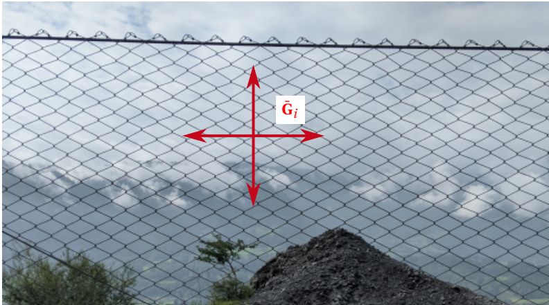
Figure 3.2: Orientation of \tilde{\mathbf{G}}_i in the wire mesh. Photograph taken in Walenstadt, Switzerland. The respective Young's Moduli for each direction are obtained from tensile tests.
