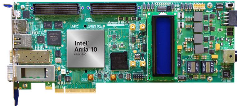
Figure 2.7.: An FPGA development kit with functional flexibility suitable for hardware prototyping
