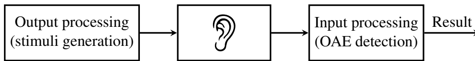
Figure 2.11: High-level signal processing components of an OAE measurement, during which stimuli generation is mostly independent of the input processing.
