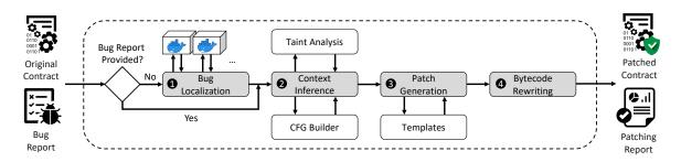
**Figure 8.6:** Overview of ELYSIUM's architecture. The shaded boxes represent the four main steps of ELYSIUM.
