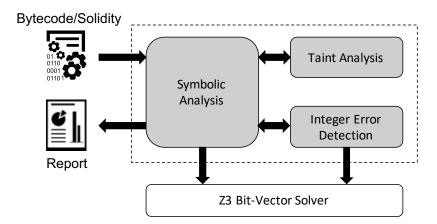
**Figure 3.7:** Architecture overview of OSIRIS. The shaded boxes represent its main components.
