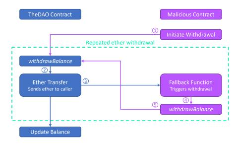
Figure 1.1: A visual example of the DAO reentrancy attack.
