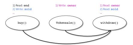
**Figure 4.3:** A dependency graph illustrating read-after-write (RAW) data dependencies contained in Figure 4.1. A node represents a smart contract function while an edge indicates a RAW dependency between two functions.
