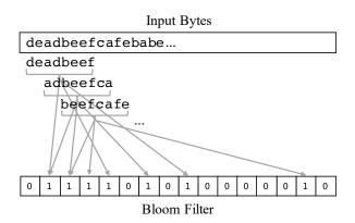
Figure 7.3: An example on how transaction input bytes are mapped into a bloom filter.
