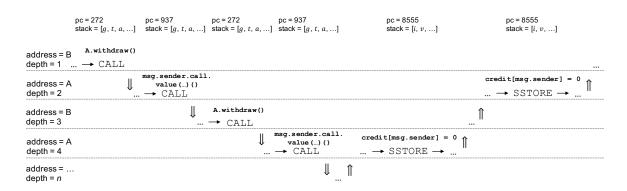
**Figure 9.4:** Execution example of a reentrancy attack, where the stack values g (gas), t (to), a (amount), i (index) and v (value) represent the respective parameters passed to the instructions during execution. A control flow relation is depicted using  $\Rightarrow$ , while  $\rightarrow$  depicts a follows relation.
