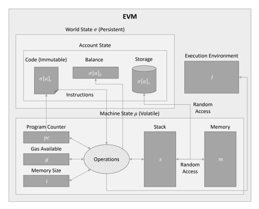
Figure 2.7: Architecture of the Ethereum Virtual Machine.
