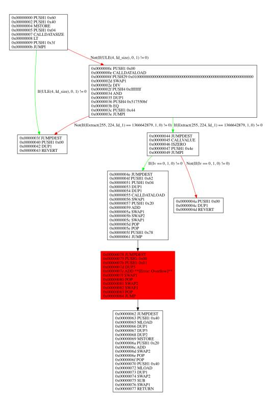
**Figure 3.8:** A representation of the control-flow graph that OSIRIS produces for Figure 3.9. The basic block highlighted in red indicates the location where an overflow may occur.
