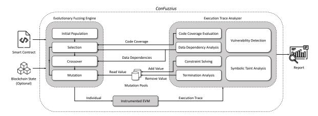
**Figure 4.4:** Overview of CONFUZZIUS's hybrid fuzzing architecture. The shadowed boxes represent the three main modules and form together a feedback loop.
