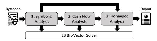
**Figure 6.10:** An overview of the analysis pipeline of HONEYBADGER. The shaded boxes represent the main components.
