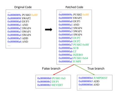
**Figure 8.8:** An example on bytecode rewriting, where a guard is added to an unguarded ADD instruction using the *integer overflow (addition)* patch template.
