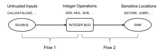
**Figure 3.6:** An integer bug is reported as valid if it originates from a source (i.e., untrusted input) and flows into a sink (i.e., sensitive location).
