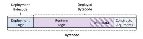
Figure 2.10: An illustrative example of the anatomy of Ethereum bytecode.
