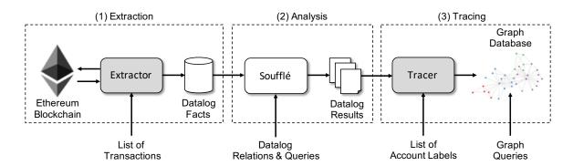
**Figure 5.1:** Architecture of HORUS. Shaded boxes represent custom components, whereas boxes highlighted in white represent off-the-shelf components.
