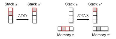
**Figure 5.3:** The example on the left depicts the propagation of taint via the ADD instruction, where the result pushed onto stack s' becomes tainted because the second operand on stack s was tainted. The example on the right depicts the propagation of taint via the SHA3 instruction, where the result pushed onto stack s' becomes tainted because the memory m was tainted.
