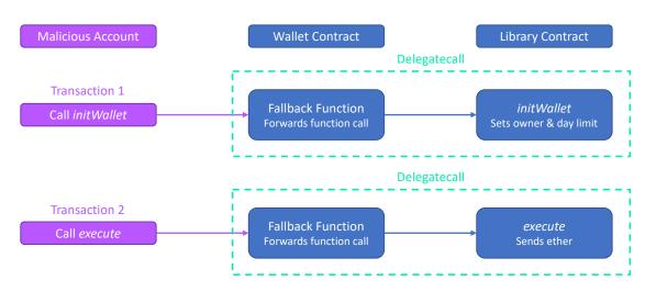
Figure 1.2: A visual example of the first Parity wallet attack.
