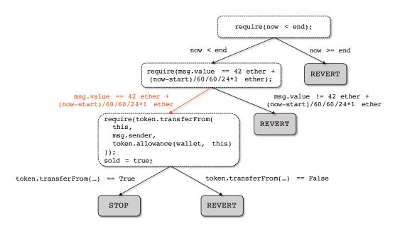
Figure 4.2: CFG of the function buy(). Complex path conditions are highlighted in red.
