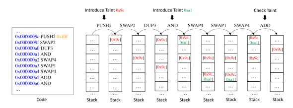
Figure 8.7: An example on the usage of taint analysis to infer integer types from bytecode.
