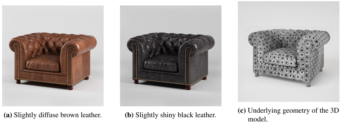
Figure 2.7: A sample high-quality CAD model of an armchair [31] that contains realistic BRDF materials and high geometric fidelity. CAD models allow easy manipulation of appearance and geometry.
