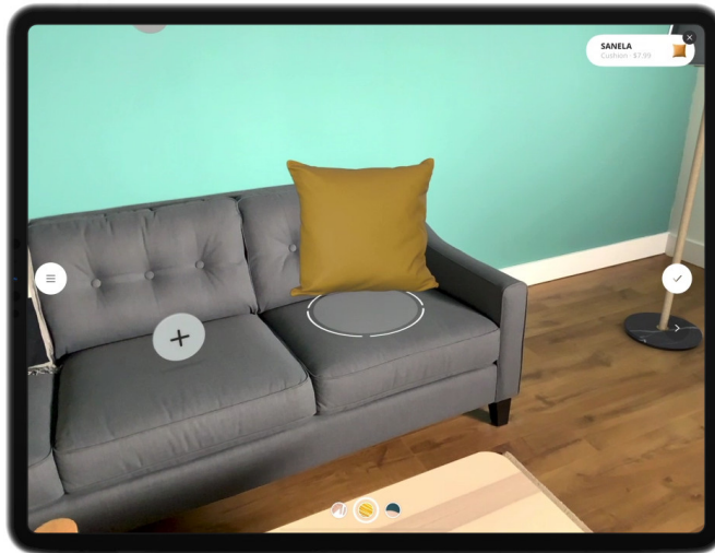
Figure 2.5: Placement of a virtual object (pillow) on the sofa with an iPad [25]. Wrong geometry estimate will cause unrealistic contact points with the sofa and bears the risks of a deficient user experience.
