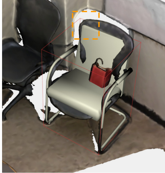
Figure 2.11: This overlay demonstrates the difficulty of shape retrieval and correspondence finding. On a high level, both chairs are very similar to each other. Low-level geometric features differ drastically, however. For example, to reliably describe the corner in the orange box both geometric and semantic features must be considered.
