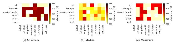
Figure 7: Absolute relative error illustrating the achieved precision of the three models (i.e., minimum, median, and maximum) on the NetFPGA SUME. White parts of the heatmaps correspond to the training set; thus, the error is always 0%.
