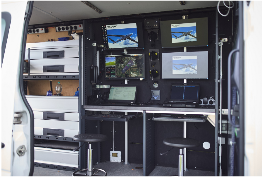
Figure 5 – Ground Control Station prepared for operations. Flight Test Operator's place on the left and Flight Test Engineer's on the right.
