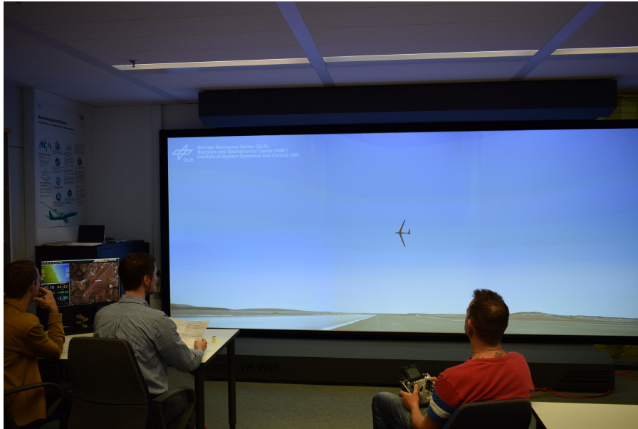
Figure 8 – Pilot and operations training setup using the flight simulator environment SimVis [29].
