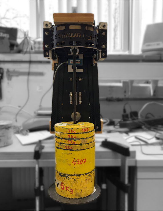
Fig. 6 Thrust measurement system is mounted vertically during the calibration.
