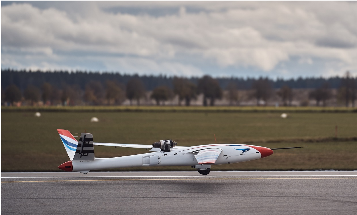
Fig. 1 T-FLEX Subscale flight demonstrator during landing phase.
