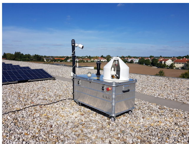
Figure 5. Image of the new enclosure system on the roof of a school at our southern site, Taufkirchen. The system includes, inter alia, the newly designed rotating cover, the lightweight aluminum case, the solar radiation sensor and a surveillance camera attached to a post.
