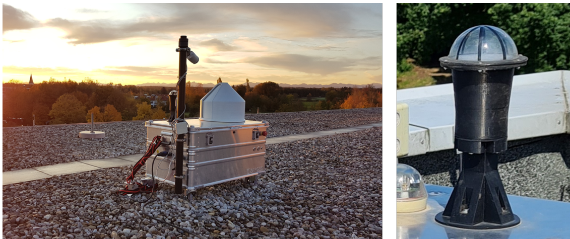
Figure 2.1.: Photos of the enclosure system: Left: enclosure system at sunrise on the roof of a school in Taufkirchen, Germany. Right: Close-up of the direct solar radiation sensor.
