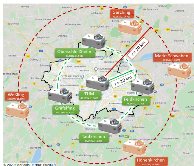
Figure 8. Map of the greater Munich area together with the two different sensor network setups that have been implemented. The urban area itself (indicated by the black border) is largely contained within the inner green dashed circle in the center, which represents the current setup of the stationary network. The light red shaded sensor systems, together with the center station, represent the setup during our 2018 summer campaign. Both setups are characterized by a center station and a station in each compass direction to measure the inflow and outflow of GHG concentrations under arbitrary wind conditions. Map data are from © Google Maps.
