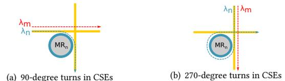
Figure 1: Working mechanism in CSEs
