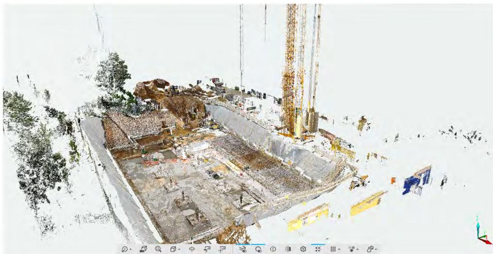
Figure 5.7: Point cloud of laser-scanner after referencing
