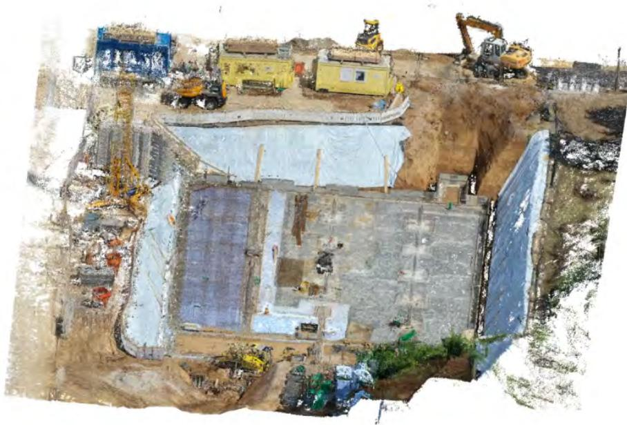
Figure 5.9: Point cloud created of drone
