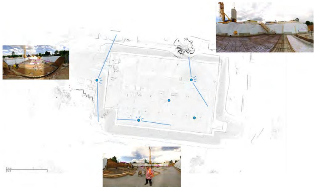
Figure 5.6: Five-point scan with Faro X130
