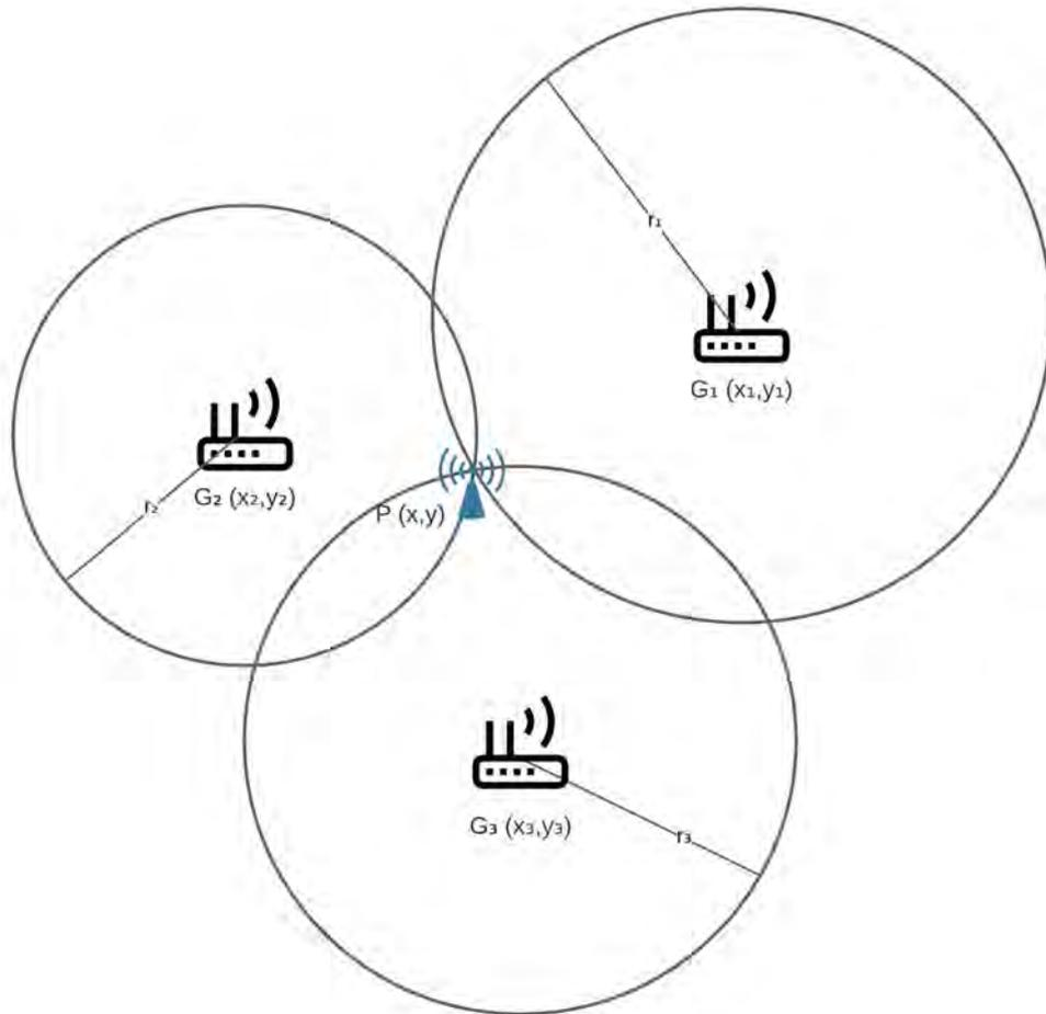
Figure 4.2: Triangulation method
