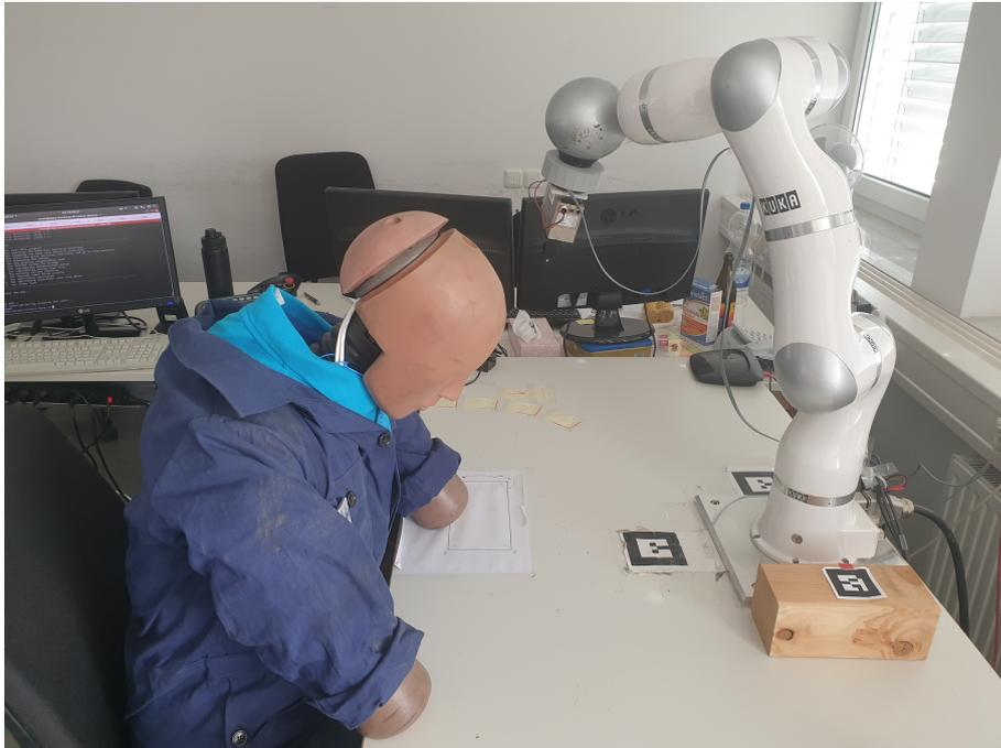
Figure 3.2: Dummy for collision sample recording.
