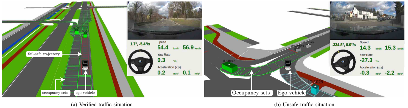
Fig. 19. Snapshots of intervention study. (a) The verification successfully computed a fail-safe trajectory (red regions). (b) Priority traffic rules are not yet implemented in the environment model. The ego vehicle cannot compute a fail-safe trajectory, since the green vehicle is predicted to turn left, merging into the ego vehicle's lane.
