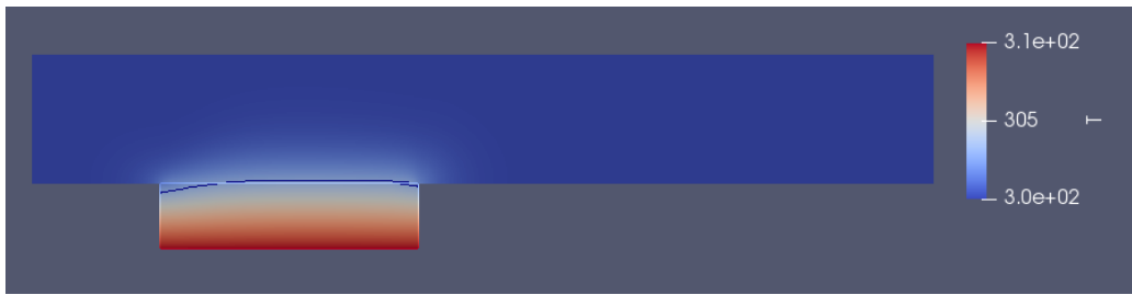
(a) Coupled flow over heated plate, fluid simulated by openFoam and solid simulated by Elmer
