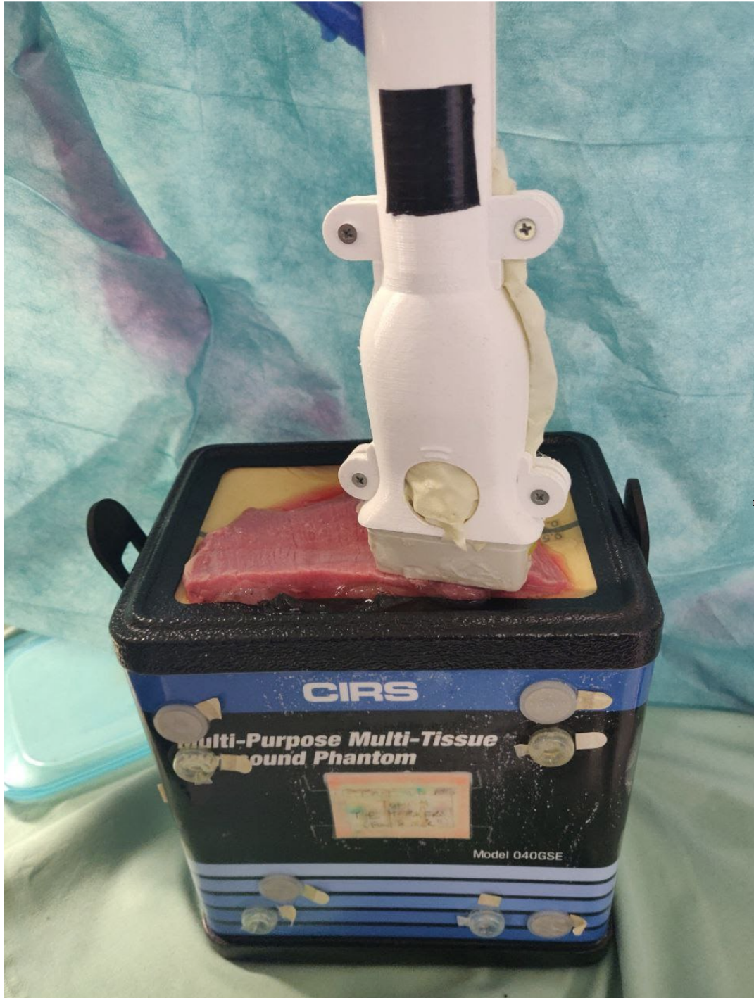
Fig. 5.3. The experimental setup of the CIRS phantom acquisition can be seen above. A porcine steak was placed between the transducer face and the CIRS calibration phantom to serve as an aberration screen.
