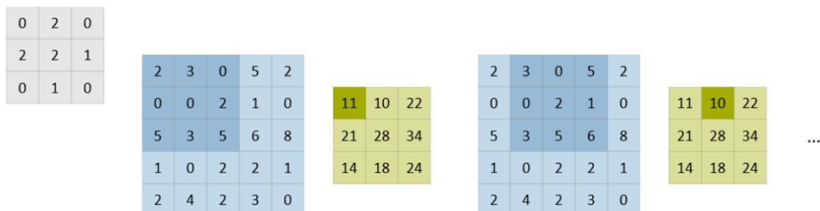
Figure 3: Convolution example: filter (gray) slides over matrix (blue), dot product is calculated at each position and written into the feature map (green) at the corresponding position (adapted from: Dumoulin and Visin 2016)
