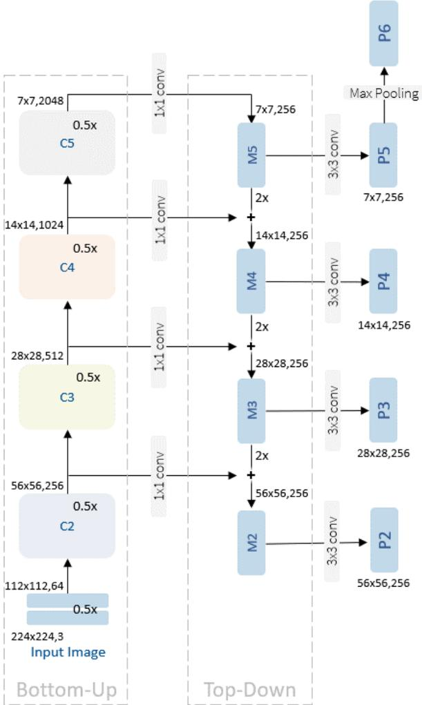
Figure 16: Feature Pyramid Network (FPN) based on ResNet-50 as Bottom-Up Backbone and Top-Down Upsampling for generating feature maps of different size (adapted from: Lin et al. 2017a; Hui 2018; Fractal AI@Scale Research Group 2019)
