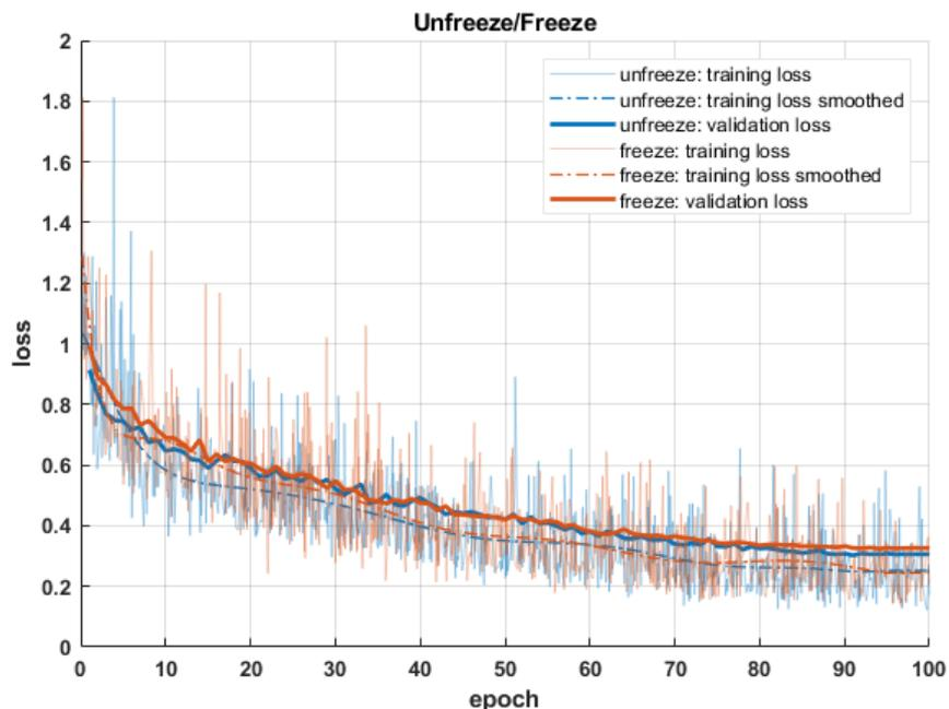
Figure 45: Training and validation loss for freezing/unfreezing the backbone: blue: unfrozen backbone, orange: frozen backbone; training losses smoothed by 12<sup>th</sup> degree polynomial for better comparison
