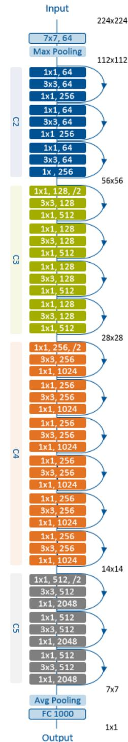
Figure 15: ResNet-50 convolutional layers (with filter size) grouped in blocks by residual connections and arranged into four stages (C2 - C5), numbers in black give the size of the output after each stage (adapted from He et al. 2016; Ankit 2019)
