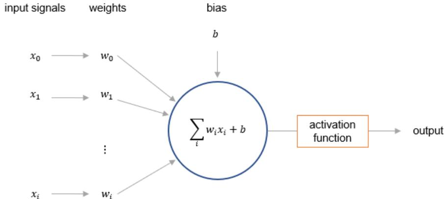
Figure 1: Mathematical model of a neuron (adapted from: Li et al. 2021)
