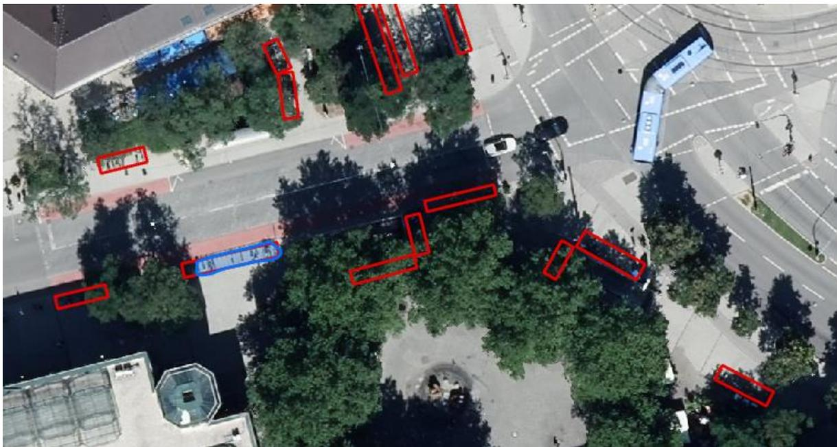
Figure 57: Detected bike parking facility at Rotkreuzplatz in 2017 imagery with RGB+nDSM; blue: detected object; red: labeled parking facilities (Image source: Landeshauptstadt München 2020)
