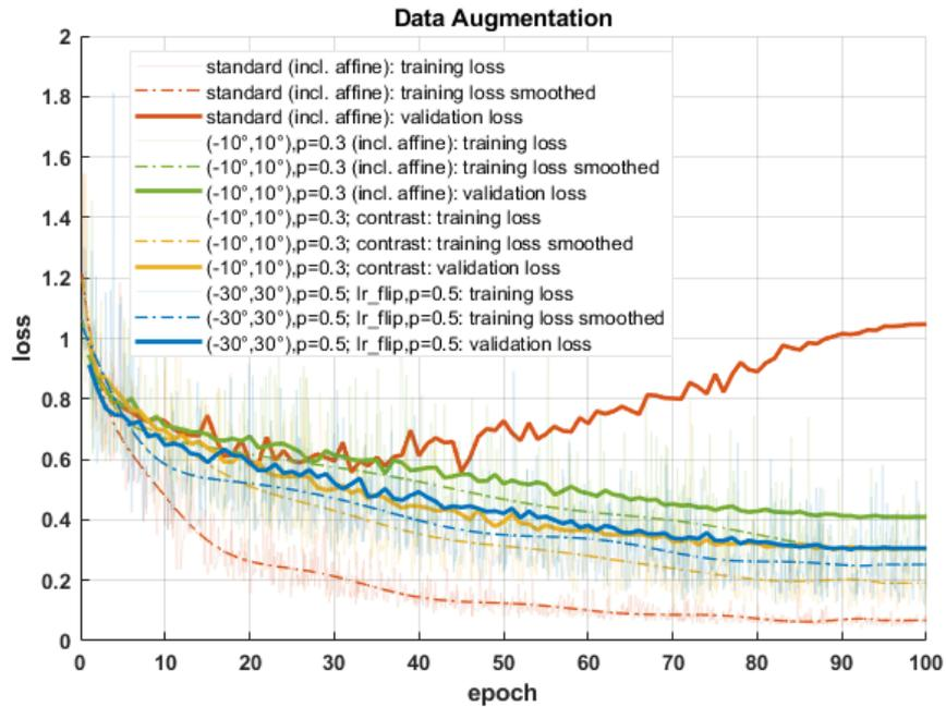
Figure 44: Training and validation loss for different data augmentations: orange: default, green: rotations  $\pm 10^\circ$ , yellow:  $\pm 10^\circ$ , contrast, blue:  $\pm 30^\circ$ , left-right flips; training losses smoothed by 12<sup>th</sup> degree polynomial for better comparison
