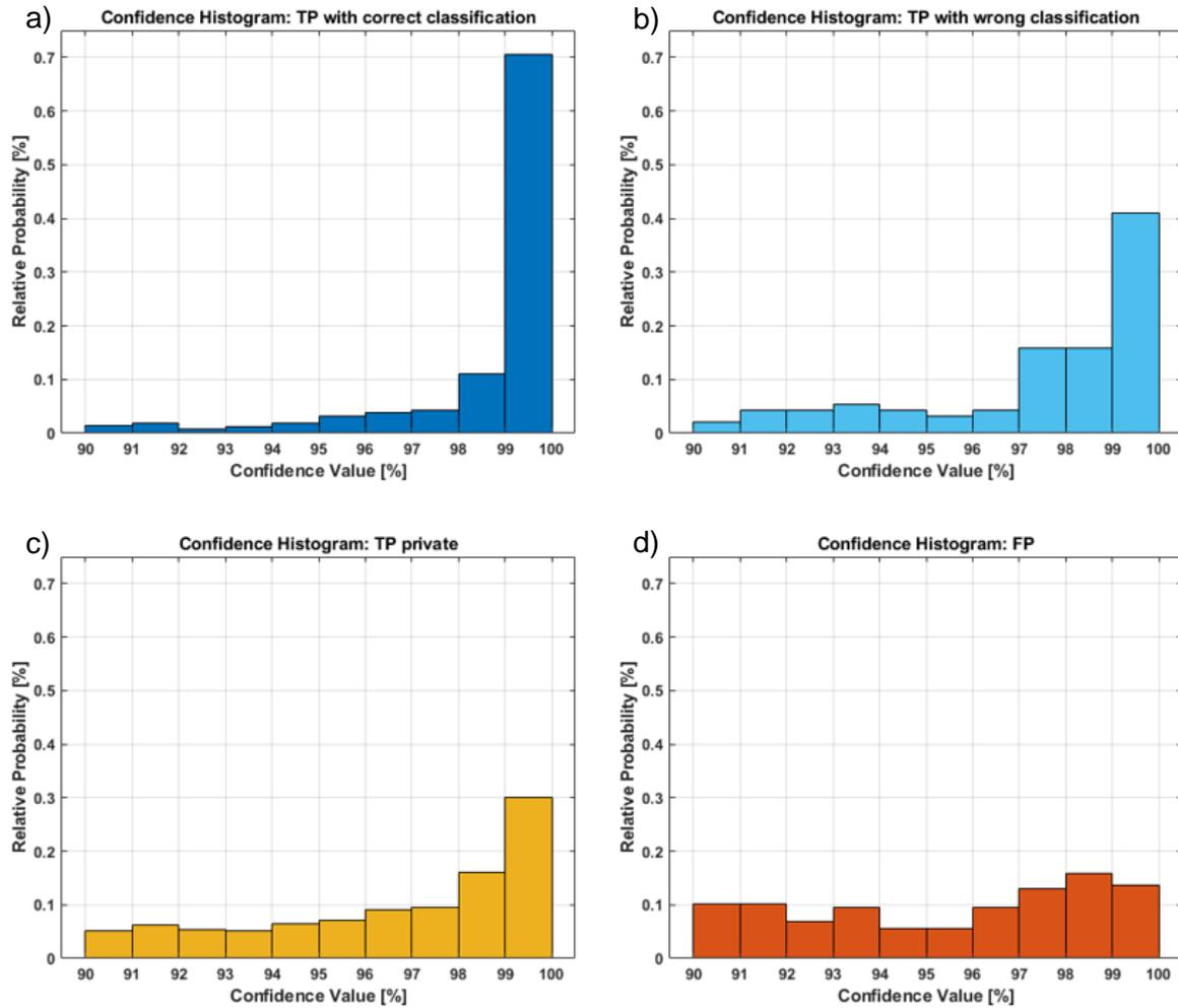
Figure 53: Histograms for confidence value distributions; a) TPs that are correctly classified; b) TPs that are wrongly classified; c) TPs on private areas and not in ground truth data; d) false positive detections
