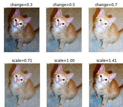
Figure 39: Brightness (top) and contrast (bottom) changes (Source: fast.ai 2021)
