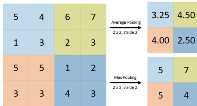
Figure 4: Examples of Average and Max Pooling with a  $2 \times 2$  filter and a stride of 2 (adapted from: Li et al. 2021)
