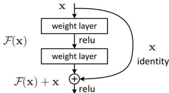
Figure 5: Residual Connection Block (He et al. 2015)
