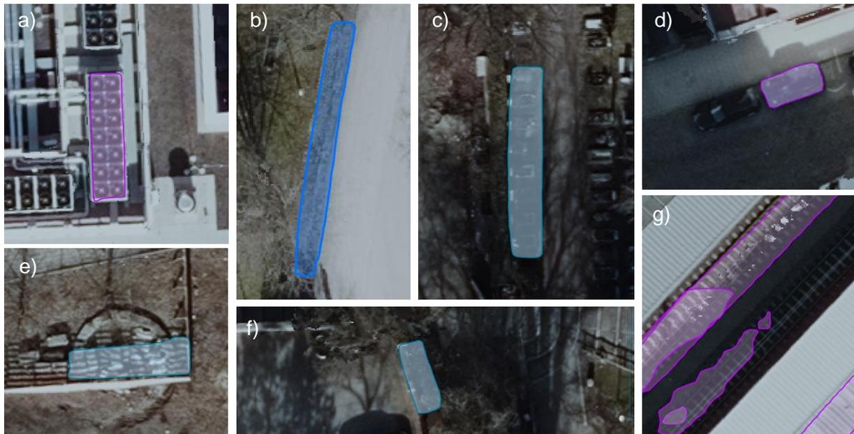
Figure 52: Examples for false positive detections: a) roof (Willy-Brandt-Platz, with RGB); b) groundclutter (Preysingstr., with RGB+nDSM); c) cemetery (Friedhof Sendling, with CIR); d) dark car (Volkartstr., with RGB); e) shadow pattern (Kidlerplatz, with CIR); f) bush (Kidlerplatz, with CIR); e) tracks and roof (Ostbahnhof, with RGB) (Image source: Landeshauptstadt München 2020)
