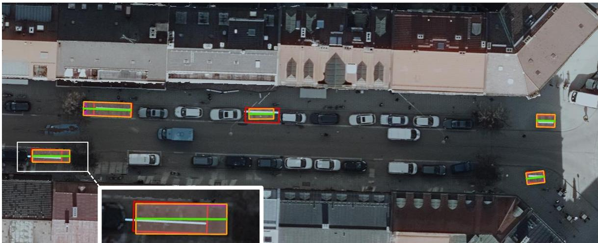
Figure 61: Application of the new *Detected Objects to Lines and Rectangles* tool (Weißenburger Straße) incl. zoom detail; light blue: bike racks in *Fahrradstaender\_bis\_2019.shp*; red: ground truth labels; pink: detected object masks (with RGB); orange: new bounding rectangle; green: new line (Image source: Landeshauptstadt München 2020)
