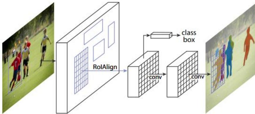
Figure 14: Simplified representation of the Mask R-CNN architecture (Source: He et al. 2017)
