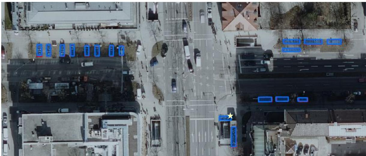
Figure 56: Detected bicycle parking facilities with RGB+nDSM in Laim (Gotthardstr./Friedenheimer Str.): red: labeled parking facilities; blue: detected parking facilities; star: facility not labeled but detected and property of the LHM
