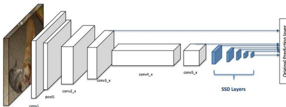
Figure 10: Simplified representation of the Single Shot Detector architecture (Source: ESRI 2021f; adapted from Liu et al. 2016)
