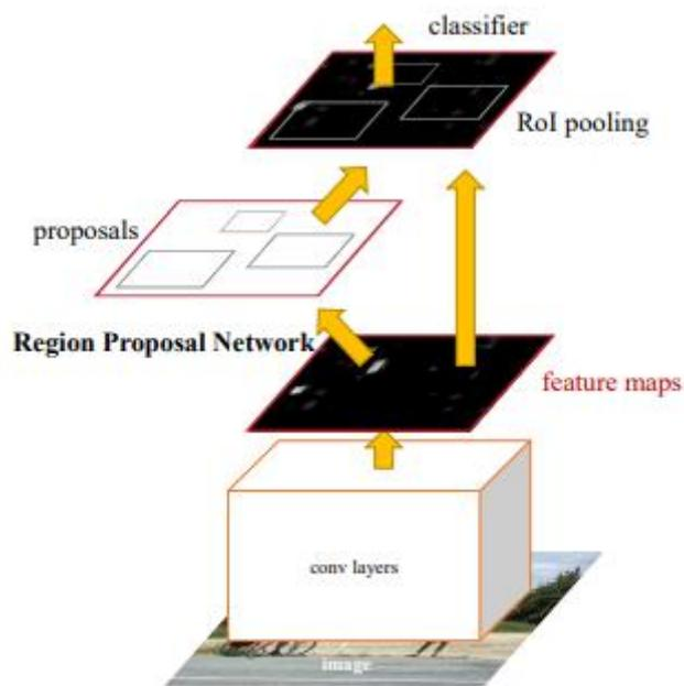
Figure 13: Simplified representation of the Faster R-CNN architecture including Region Proposal Network (Source: Ren et al. 2015)
