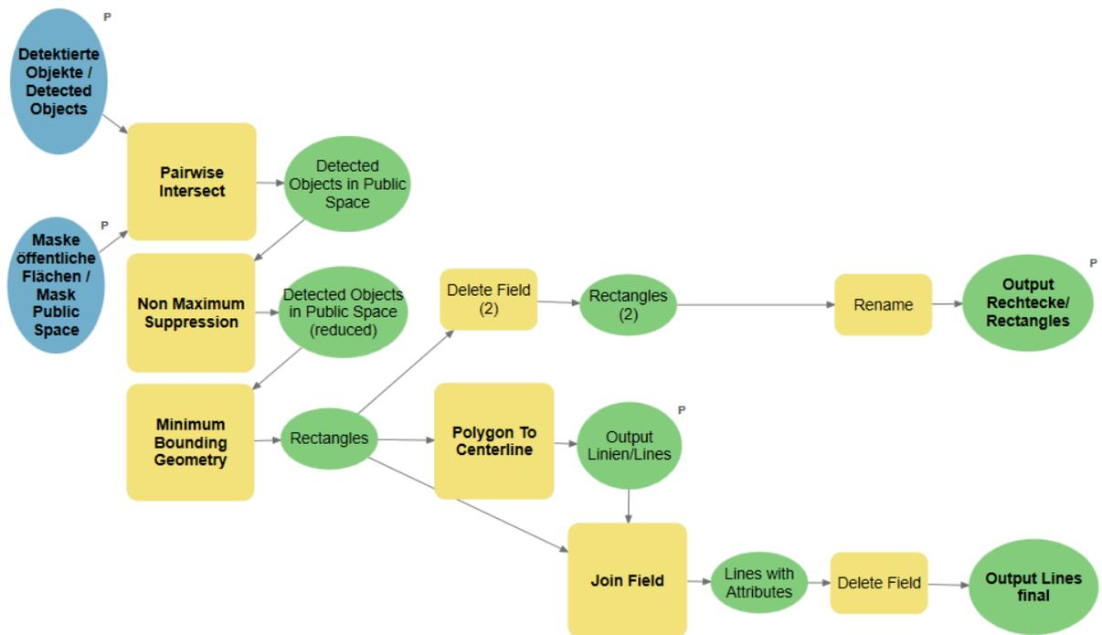
Figure 50: Postprocessing steps in Model Builder: blue: input feature classes; yellow: calculations; green: intermediate results/final results
