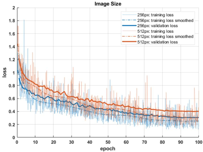
Figure 40: Training and validation loss for different image sizes: blue: 256 px x 256 px, orange: 512 px x 512 px; training losses smoothed by 12<sup>th</sup> degree polynomial for better comparison
