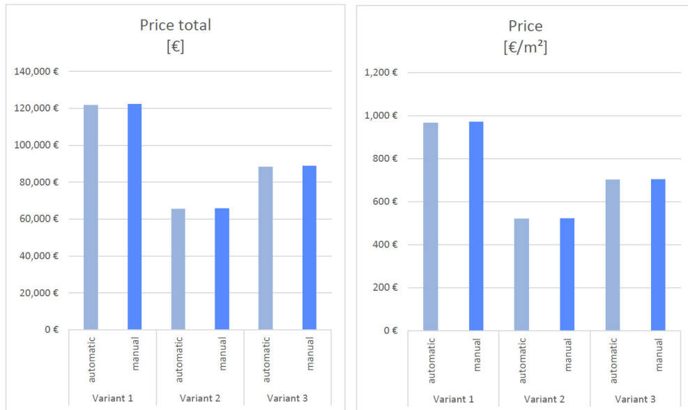
Figure 4.3: LCC calculation results for variant 1 and 2. (1) Total and (2) per m 2 net gross area. Graphs are displayed in full size in Appendix 3 + 4.
