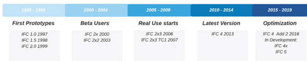
Figure 2.4: IFC Releases since 1995 (Based on BUILDINGSMART, 2021 and D. T. LIEBICH and WEISE, 2017)
