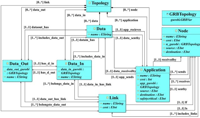
Fig. 2. The metamodel containing elements used for creating topology instances, generating constraints, and solving architectural optimization problem.
