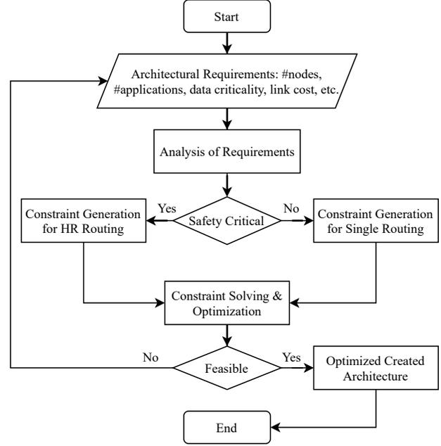
Fig. 1. The system architecture to create homogeneous redundant E/E architectures.
