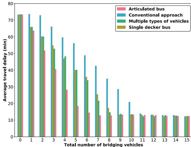
FIGURE 4. The average travel delay with different approaches.
