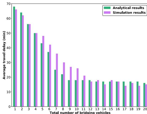
FIGURE 7. The average travel delay for optimization and simulation.
