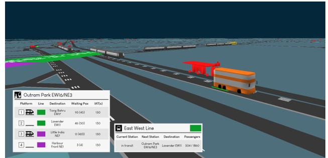
**FIGURE 5.** Screenshot of the CityMoS environment showing bus and MRT operation. Passenger information for each station, stop, train, and bus can be displayed.
