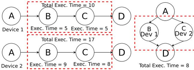
**Fig. 3.** Co-exec. leads to a gain even if sub-optimal hardware is chosen.
