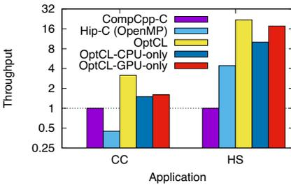
Fig. 6. Throughput of SYCL applications on the iCPU-GPU system.
