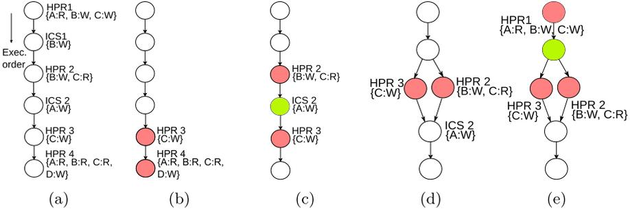
**Fig. 2.** DAG generation. (a) Original DDG (b) Processing HPR3&4 (c) Proc. HPR2&3 w. ICS2 (d) Parallelising HPR2&3 (e) Proc. HPR 1, 2&3 w. ICS1
