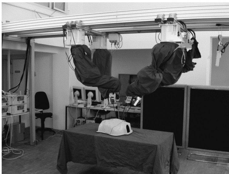
Figure 1. EndoPAR system. The four-ceiling mounted robots are shown with an artificial chest on the operating table to test tele-operated and autonomous surgical procedures. Three of the robots hold laparoscopic gripper instruments, while the fourth manipulates an endoscopic stereo camera that provides the surgeon with images from inside the operating cavity. The size of the operating area (including gantry) is approximately 2.5 m × 5.5 m × 1.5 m and the height of the operating table is approximately 1 m.
