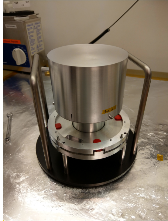
(b) The support structure designed for the storage of the n-type segmented BEGe. The detector is located inside the aluminum cylinder, which serves as infrared shield when installed in a cryostat.
