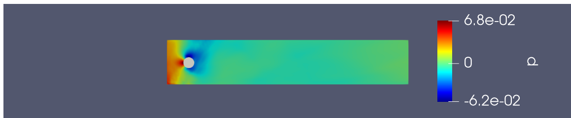
(a) Pressure distribution with SELU activation Function
