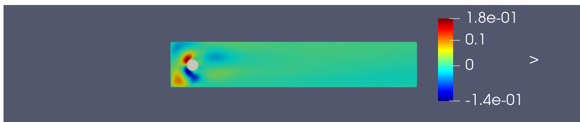
(a) Velocity v with SELU activation Function
