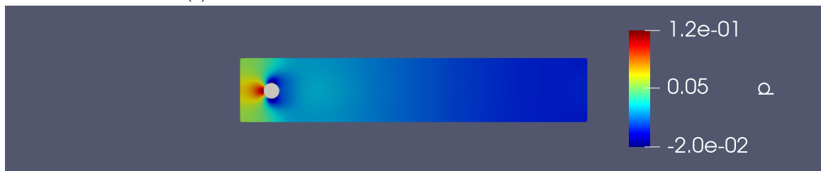
(b) Pressure distribution with Swish Activation Function
