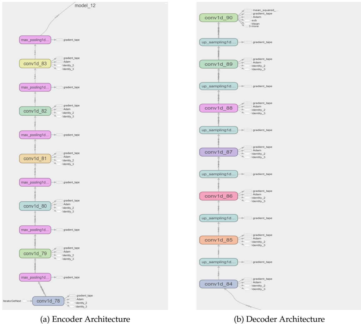
Figure 4.2: The figure shows the architecture of the constructed encoder and the decoder part of the CAE. This architecture is used for both combined and separated training. The input block to the network is at the bottom and the output block is at the top. The figure is generated using tensorboard toolkit available in the tensorflow library [3].
