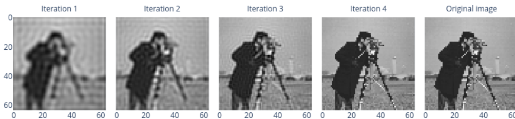
Figure 1.1: The levels of the MultiscaleGeometricHarmonicsInterpolator predicting the train image beginning with the coarsest scale.
