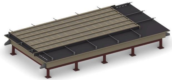
Fig 4.6. Base plate on the vibrating table
