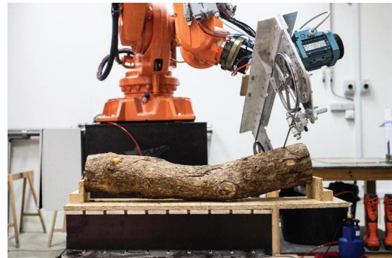
Fig. 7.4. Robotic milling of logs at Aarhus school of architecture
