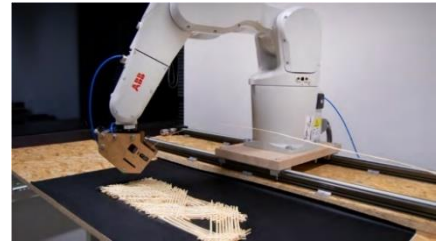
Fig. 2.12. Continuous timber fibre placement
