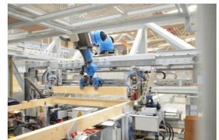
Fig. 2.8. Weinmann stud fitting station
