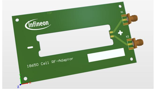
Fig. 2. Printed circuit board cell fixture with microstrip traces and SMA connectors. X1 is connected to port 1 and X2 is connected to port 2 of the VNA.
