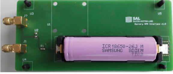
Fig. 1. Photo of the PCB used in this work. It enables 2-port shunt-through S-parameter measurement, as well as connection of SMD loads in parallel and/or series to the battery holder. The PCB's bottom layer is a solid GND plane. Underneath most of the battery holder is another GND plane on the top layer, used to connect 'Short' and 'Load' between battery plus pole (left) and GND during OSL compensation with soldered standards, see Fig. 2.
