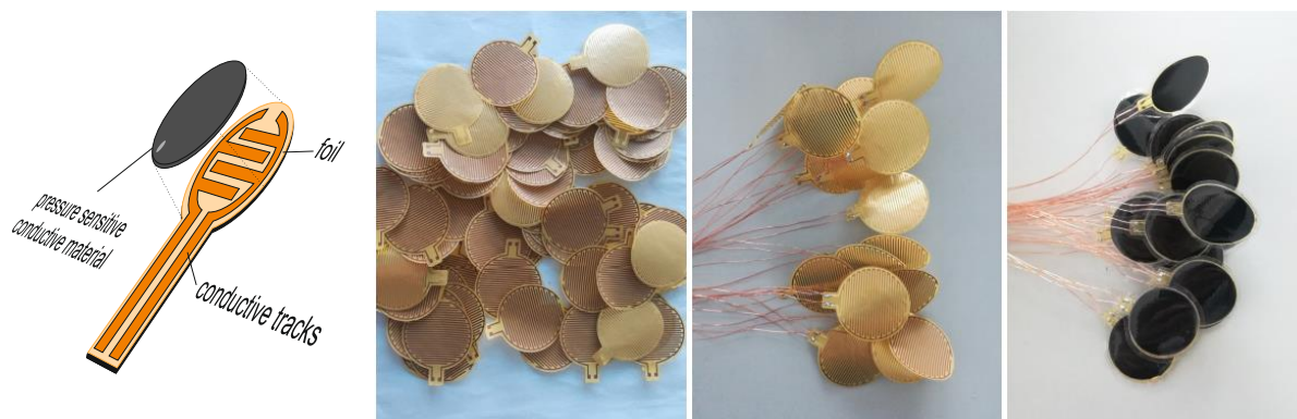
Figure 4-25 SHEMA of the pressure sensor (left) and steps of manufacturing: centre left: foils with conductive tracks; centre right: wired sensor foils; right: finished sensor with pressure sensitive conductive material layer over the foils with the conductive tracks and protective, non-conductive foils laminated on both sides of the sensor.
