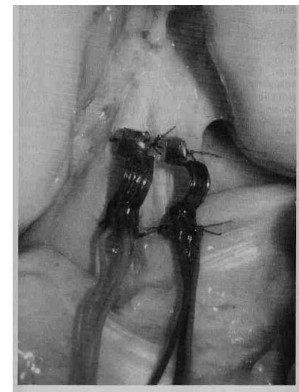
Figure 7-12 Two \Omega -transducers. One attached to each bundle of the ACL. Original source Dürselen et al. (1995), taken with permission.
