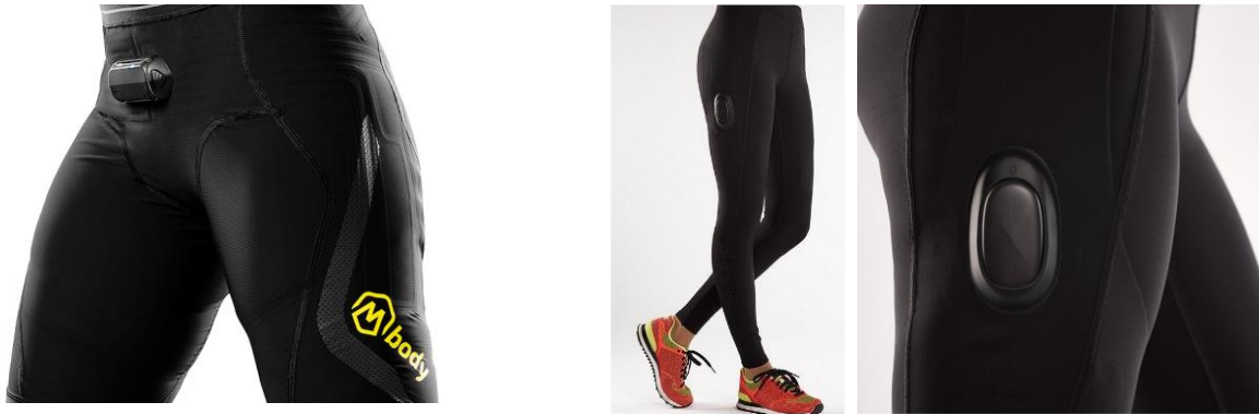
Figure 4-10 Commercially available sports garments for tracking muscle activity of the tights by Myontec (left) and Athos (right). Pictures taken from the websites www.myontec.com and shop.liveathos.com on the 21.03.2020.
