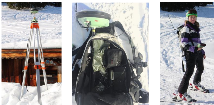
Figure 4-36 from left to right: reference station, rover and low-cost prototype in the backpack carried by the test skier, test skier
