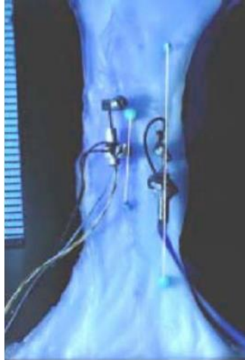
Figure 7-13 Exemplary measurement using the DVTS. Observable are local strain differences in the structures. Picture taken with permission from Lehner (2007)
