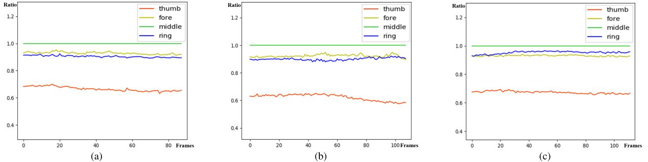
Fig. 9. Ratios of the fingers' (thumb, forefinger, middle finger, and ring finger) length to middle finger length under different light conditions. (a) Data recorded in an ideal environment. (b) Data recorded with the concurrent flashlight. (c) Data recorded in a low-brightness environment.
