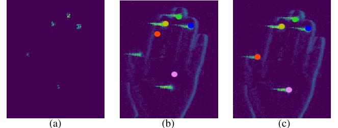
Fig. 5. Tracking results with traditional particle filter and RSTP filter. (a) Evidence map for the particle filter. (b) Tracking results of a traditional particle filter without spatial restriction. (c) Tracking results of our RSTP filter (with restriction).
