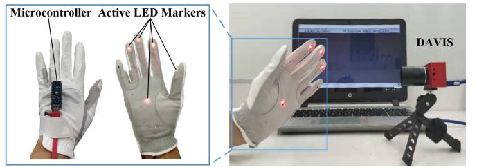
Fig. 2. Illustration of our hand gesture recognition system. A system prototype consists of an event-based neuromorphic vision sensor and an ALM glove.
