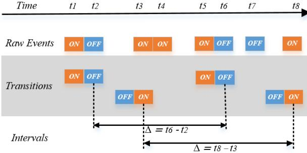
Fig. 3. Illustration of processing a sequence of raw events that occur on the same pixel within a certain temporal window. Event data processing consists of three stages: raw events, transitions, and intervals. Raw events are translated into intervals ( $\Delta$ ) via transitions, and intervals serve as robust estimators for blinking periods of ALMs.
