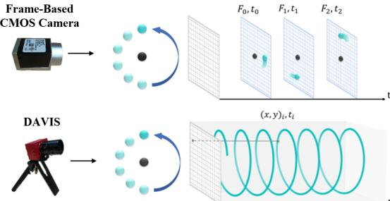
Fig. 1. Illustration of the different working principles of frame-based CMOS camera and neuromorphic vision sensor. The green ball is rotating around a black ball. Frame-based CMOS camera captures intensity values at a fixed rate, while the neuromorphic vision sensor (DAVIS) captures intensity changes asynchronously.
