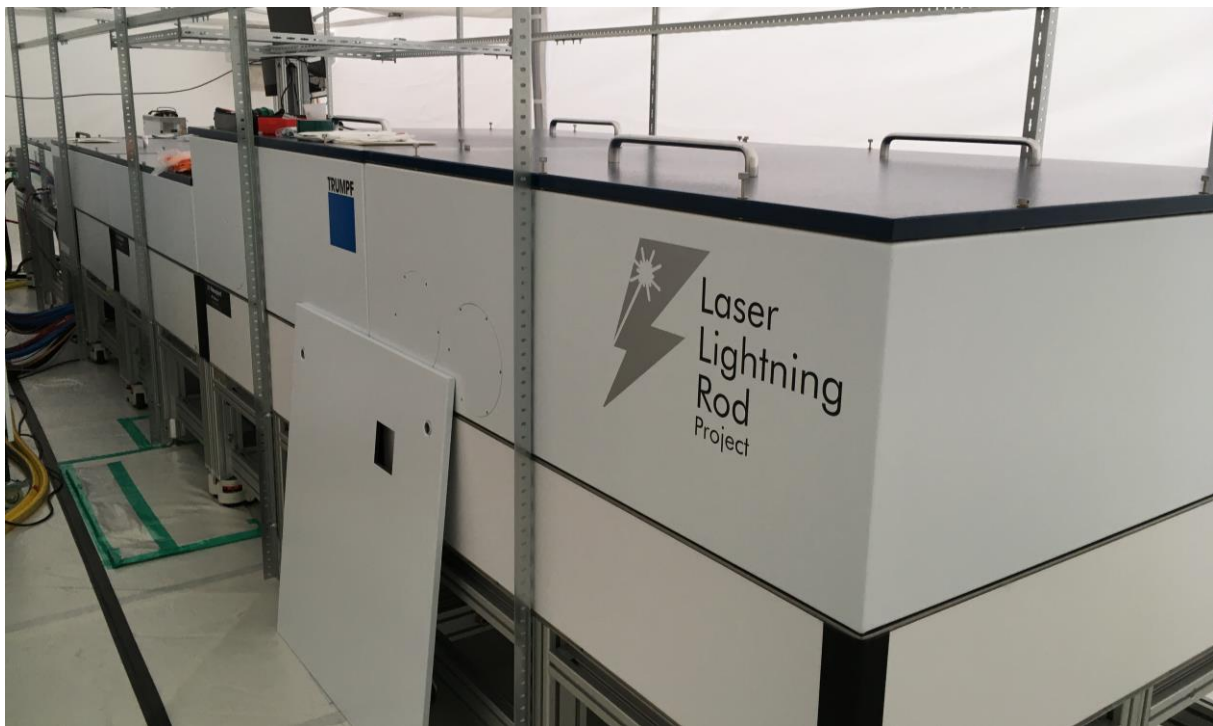
Figure 5.29: Photograph of the completed laser system used for experiments. From left to right, the regenerative amplifier, multipass amplifier, and grating compressor are visible.
