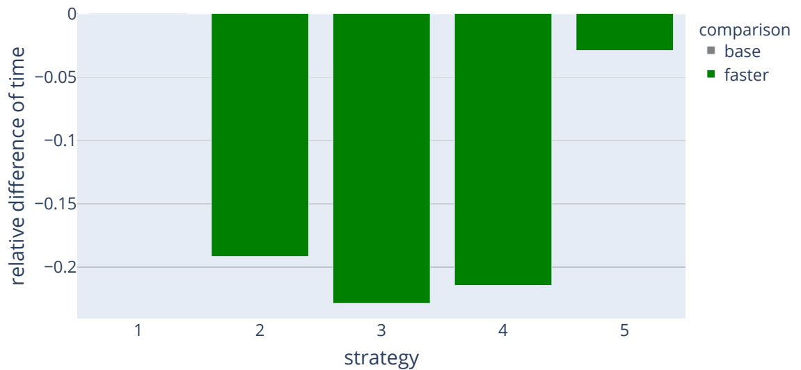
Figure 7.2.: Relative difference of total execution time of slowest scenario of several tuning-strategies. Strategies are compared to no MPI-tuning. Green bars represent faster strategies. The lower the bar, the faster the execution time.
