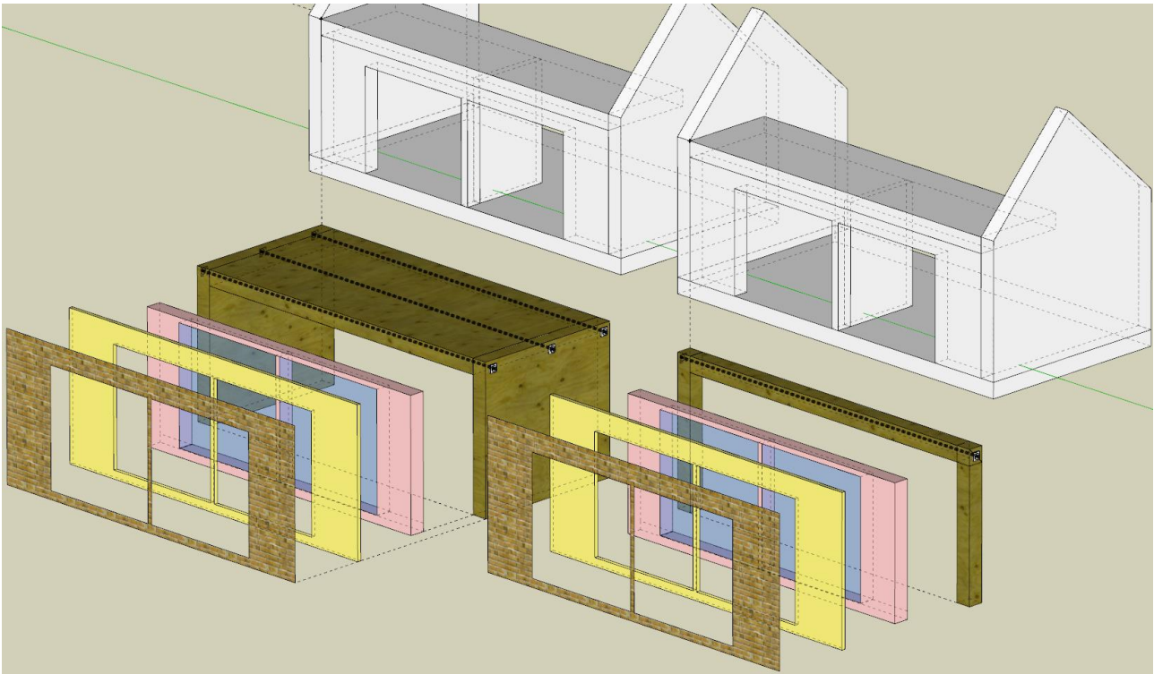
Figure 1. Overview 3D-PT-Frame (left) and 2D- PT-Frame both façade element infill, insulation layer and façade cladding [own model].
